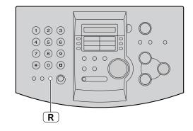
If your unit is connected to a PBX, pressing  $\boxed{\mathbf{R}}$  allows you to access some features of your host PBX such as transferring an extension call.
